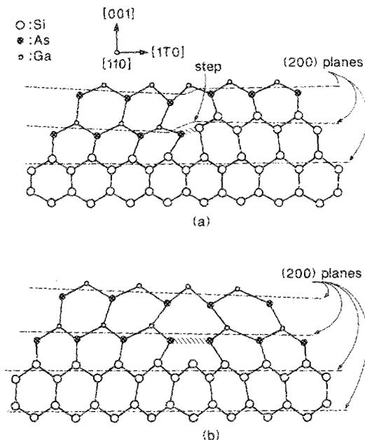
FIG. 3. Dislocation microstructure constructed from Figs. 1 and 2. Note that the dash lines in (a) and (b), representing the (200) planes, show characteristics similar to those in Figs. 1 and 2, respectively.
